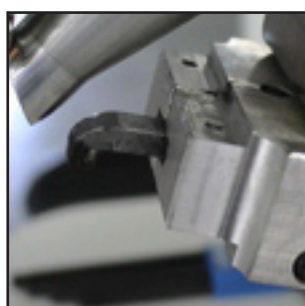
13_ Now the head of the machine appears you without shaving thread cutter and cover.
