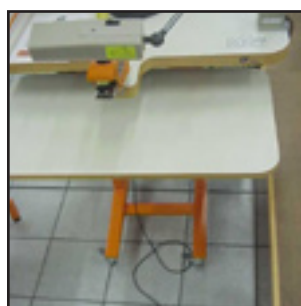
20_ We suggest to use the pedal only on small garments where the photocell cannot recognise the fabric.
