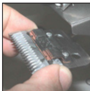
16_ Re-assemble the shaving thread cutter combining the 2 locking screws holes .
